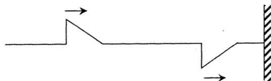
Two pulses of the same shape travel along a stretched string with one end fixed to the wall as shown above. Which of the following can be the resultant waveform at different instants later?
