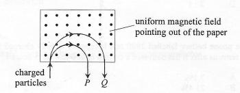
P and Q are two particles carrying the same amount of charge but of different masses. They travel with the same speed and enter a uniform magnetic field pointing out of the paper as shown. Semi-circular paths with different radii are described before they emerge from the field. Which descriptions below are correct?
