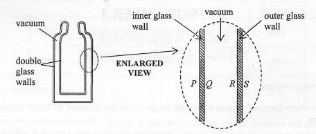
The figure shows a vacuum flask with double glass walls for keeping liquids cold. P, Q and R, S are the glass surfaces of the inner and outer glass walls respectively. Which two surfaces are usually coated with silver?
