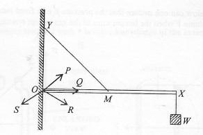
A uniform light rigid rod OX is hinged smoothly to a wall at one end O. Its mid-point M is connected by a light inextensible string to a point Y directly above O while a weight W is suspended from the other end X of the rod as shown. Rod OX remains horizontal. The reaction force acting on the rod due to the wall is along the direction
