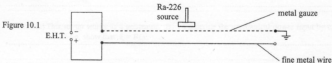
A spark counter consists of a fine metal wire mounted a few mm beneath an earthed metal gauze. The wire is connected to the positive terminal of an E.H.T. (Extra High Tension) supply so that a very intense electric field is set up between the wire and the metal gauze. When a Ra-226 source is brought near the gauze, sparks giving out flashes of light and crackling sound are produced at irregular intervals.
