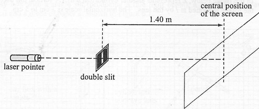
Figure 7.1 shows a set-up for measuring the wavelength  $\lambda$  of light emitted by a laser pointer. Several bright dots of average separation about 2 mm can be seen on the screen.
