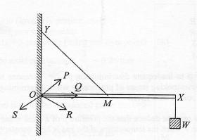
A uniform light rigid rod OX is hinged smoothly to a wall at one end O. Its mid-point M is connected by a light inextensible string to a point Y directly above O while a weight W is suspended from the other end X of the rod as shown. Rod OX remains horizontal. The reaction force acting on the rod due to the wall is along the direction
