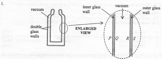
The figure shows a vacuum flask with double glass walls for keeping liquids cold. P, Q and R, S are the glass surfaces of the inner and outer glass walls respectively. Which two surfaces are usually coated with silver?
