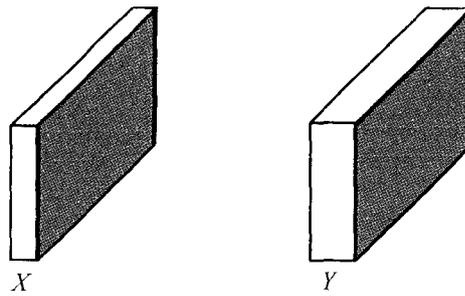
Walls  $X$  and  $Y$  having the same area are made of the same material, with  $Y$  thicker than  $X$ . If the temperature difference between the two faces of each wall is the same,  $X$  and  $Y$  have the same
