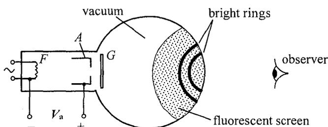
Electrons liberated from a heated filament  $F$  are accelerated by a high voltage  $V_a$  between  $F$  and anode  $A$ . The electrons then pass through a thin graphite film  $G$  and form bright and dark concentric rings on a fluorescent screen as shown. Which descriptions about this experiment are correct ?
