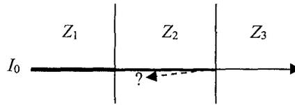
Assume that attenuation and absorption of ultrasound are negligible. What is the intensity of the ultrasound reflected from the interface between the media of acoustic impedances  $Z_2$  and  $Z_3$  ?
