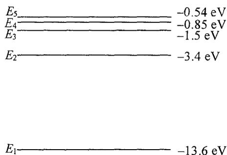
The figure shows the five lowest energy levels of a hydrogen atom. If electron transition from  $E_4$  to  $E_2$  emits a photon of blue light, which electron transition below would emit red light?
